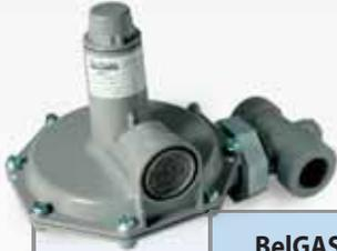
The **Type P143 Gas Pressure Regulator** from BelGAS is ideal for natural gas, air, propane and general purpose gas pressure regulation. Uses include commercial, residential and light industrial for burners and unit heaters. The Type P143 has an internal relief device and is available in the low pressure cut off – LPCO – version. The regulator is applicable to a wide range of gaseous fluids, including air, natural gas and propane. Can be used as a LP regulator.
