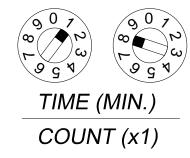
NOTE: The time (18 minutes) above corresponds to the dial setting shown for the Z-65/6.1 model with the timer range setting in the factory position (jumper on the two left pins). See Section 10.4 Timer Range Setting.
