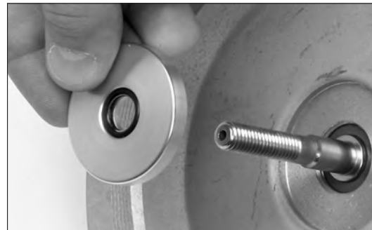
Figure 32 - Installing lower diaphragm retainer
