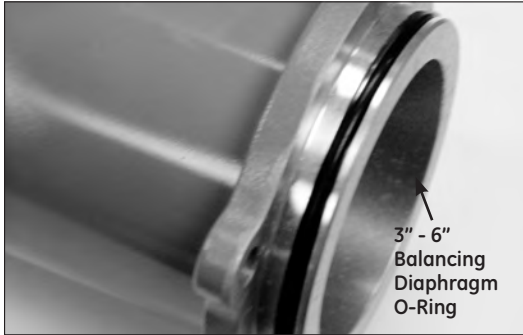
Figure 24b - Installing the balancing diaphragm o-ring on the 3", 4" & 6" FlowMax
