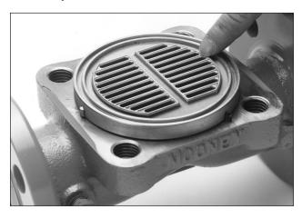
The outside "rib" on the downstream side of the throttle plate is where shutoff takes place in the Flowgrid Regulator.
