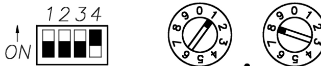
Figure 9 shown below reflects Example #1 setting of 18 pulses counted before stroking the pump.
