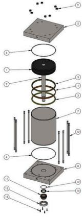
Figure 2 - RPDA Actuator Cylinder Exploded View
