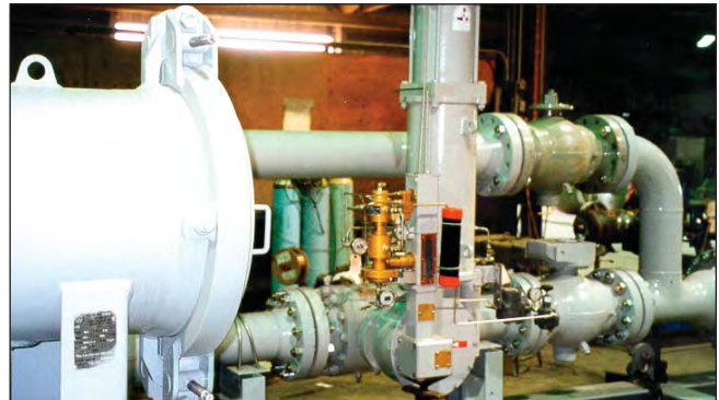
Figure 16 - Becker RPSR Actuators are ideal for Surge Control/Recycle Valves
