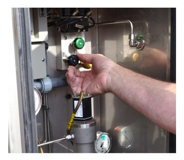
Disconnect Solenoid Vent Hoses by Pushing in on Fitting Release Ring & Pull Hose Out
