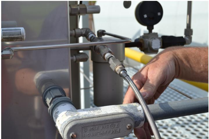
Locate the Flare in a Safe Area, Open V5 and Ignite The Flare Until The Expansion Tank Pressure reaches Zero PSIG
